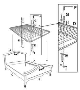
Step 2: Attach the two stands (E) onto the sprung slatted base with bolts (G), washers (H) and nuts (I), and then put the whole sprung slatted base into the bed frame.
