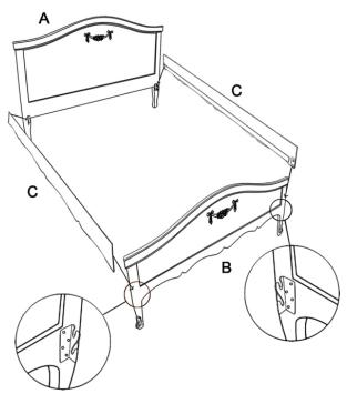
Step 1: Attach the two side rails (C) onto the head board (A) and the foot board (B) to form the bed frame.
