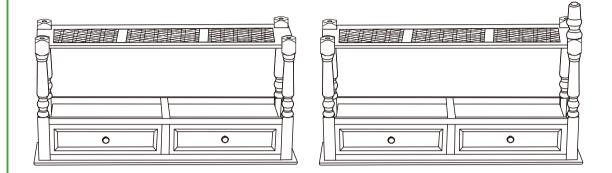
Step 3: Turn the B cane shelf upside down on the 4 long legs to make their 4 holes to fit;then insert D short legs in the the slot of shelf and long legs.
