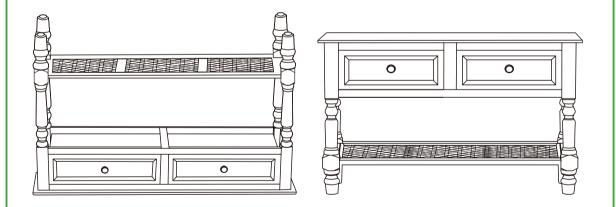
Step 4: Please repeat the other 3 short legs (D) and fully tighten fixings. Carefully turn the unit upright.
