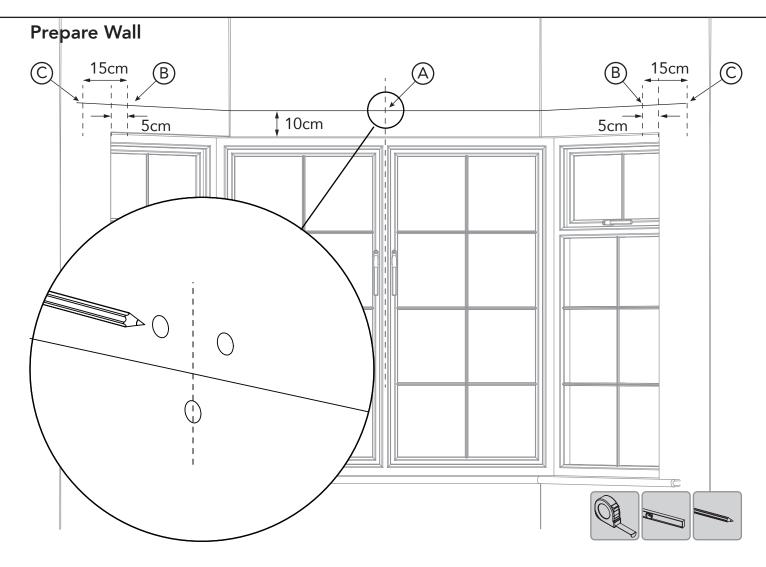
Using a tape measure and level, whilst using the wall bracket as a guide, mark the position of the brackets on the wall as shown.
