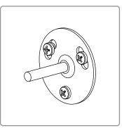
Drill holes in marked positions & fit wall plugs Screw wall plate to wall
